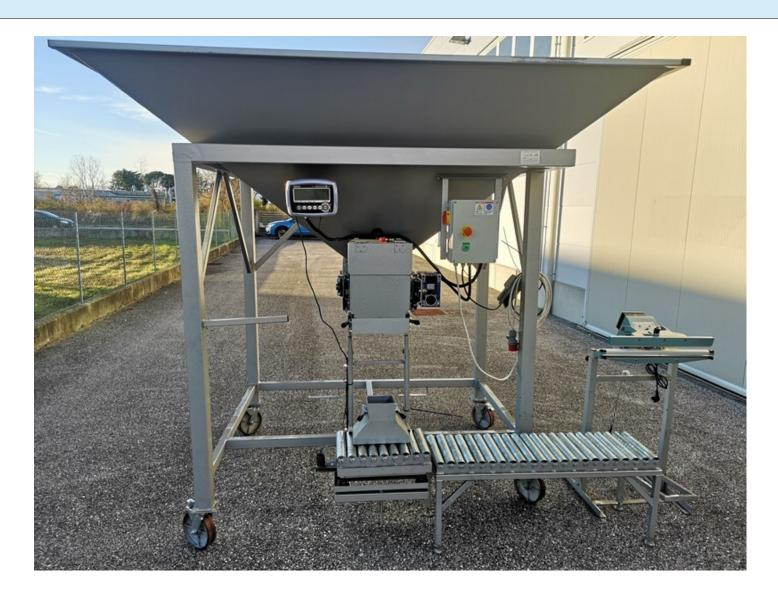
Semi-automatic bagging machine equipped with programmable precision scale.
